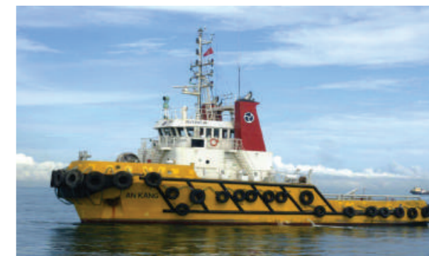
AN KANG (Towing Tug) Engines : 2 x GE 8V-228-900 rpm Gearboxes : 2 x MM W18000 NR Propellers : 2 x CPP MMS 640 Shipyard : SLS Korea
